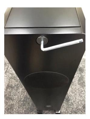
FYI, the transport screw is the ONLY screw which needs to be touched / loosened!
